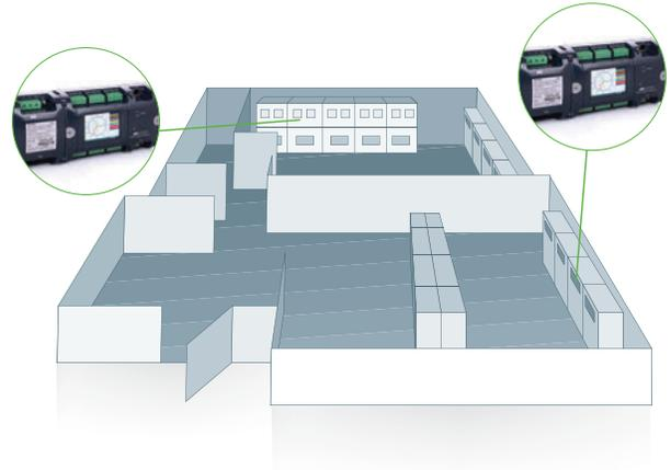
Energy consumption of data centers is constantly rising, following the increase of computing performance. Monitoring the PUE (Power Usage Effectiveness—Total Facility Energy divided by the IT Equipment Energy) is essential. According to the US DoE (Department of Energy), data centers can achieve energy savings of 20-50% by utilizing today's best practices, including "continuously monitor energy" and "monitor energy at all levels."
