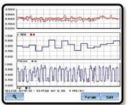
required by the load, combined with considerable variations in current occurring over a short period of time. The PowerXplorer captures flicker data per IEC 61000-4-15, which can be further evaluated using Dran-View visualization, analysis and reporting software.
