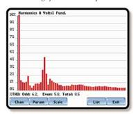
can cause small, almost imperceptible variations in performance that aggregate to effect significant long-term damage. Current harmonics generated by a source can pollute the entire power system without being effected itself. The PowerXplorer captures detailed harmonics, interharmonics and subharmonics to effectively trouble-shoot the complex problems caused by these events.
