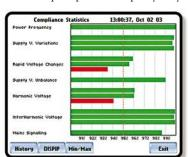
quality-of-supply standards and benchmark power quality. In an instant, the PowerXplorer provides a snapshot of over 13 key parameters, including unbalance, voltage variations and harmonics.
